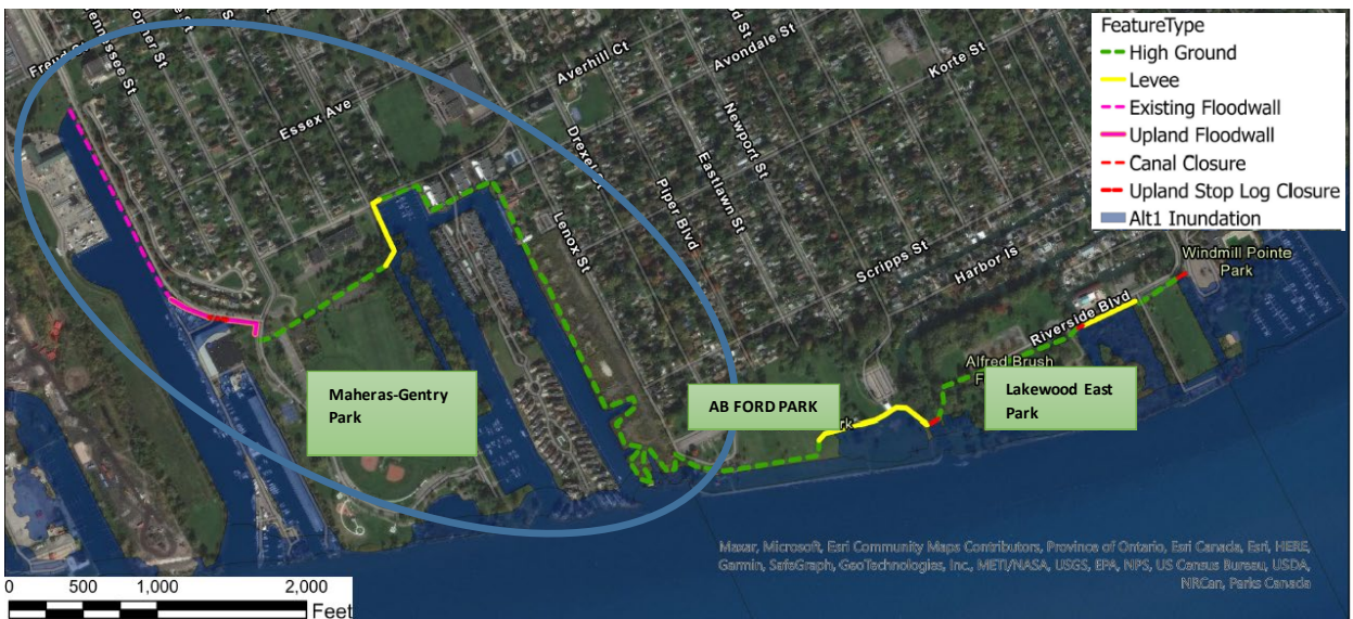
Figure 9: Conceptual alignment, Alternative 1: Closed Canal with Levees and Floodwalls Outside of Wave Run-up Zone. NOTE: Circled portion is the same for all alternatives.
