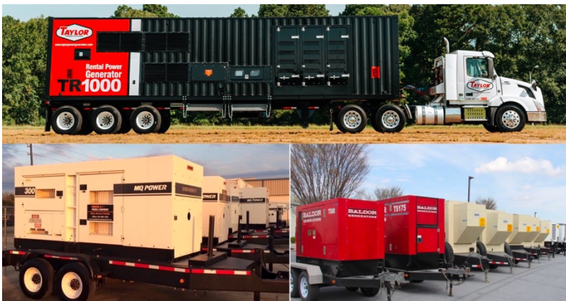
Diesel-Powered Electric Generators from GLWA Presentation
